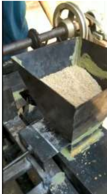
Figure 3. material funnel as a place to collect feed ingredients before mixing well
